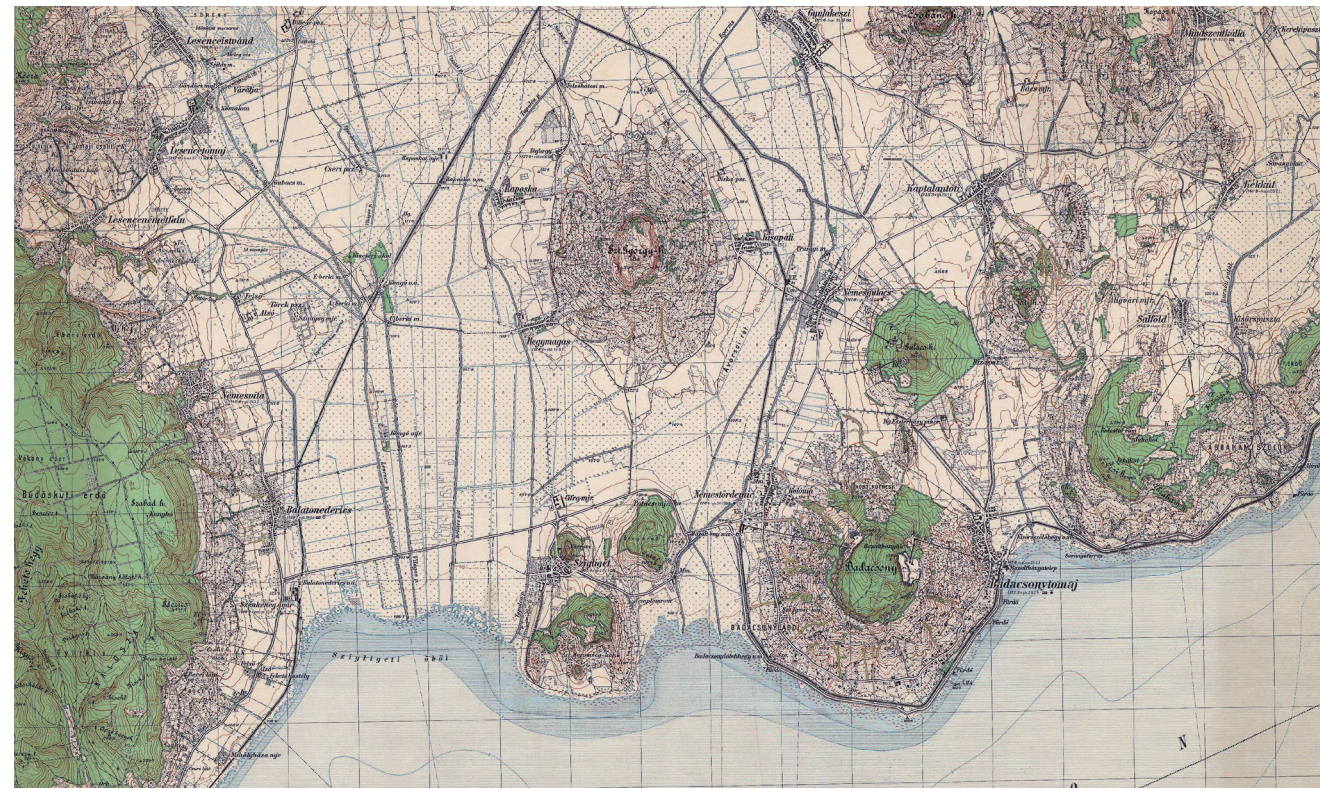
31 The area around Badacsony on a newly surveyed 1:25,000 sheet made by using aerial stereophotogrammetry (1930, detail)
